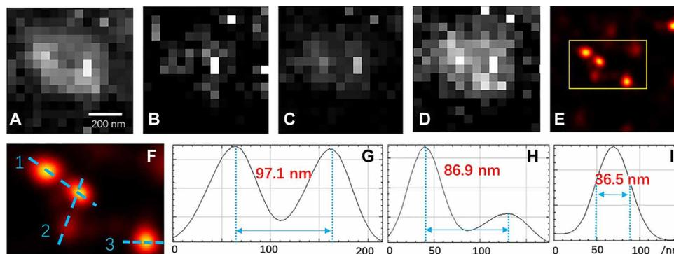
**Fig. 5. SNAC-MG reconstruction for PMMA-QD films.** (A to D) Optical images of a PMMA-QD film pumped with four SPs in a period. (E) Reconstructed image based on SNAC-MG. (F) Zoomed-in image of the yellow box in (E). Three blue dashed lines mark two adjacent points for analysis. (G to I) Profile of nos. 1, 2, and 3 dashed lines in (F), respectively.
