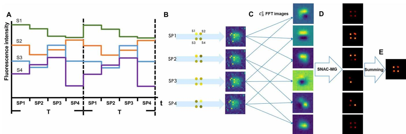
**Fig. 2. Multiple periodical excitation and image processing.** (A) Four adjacent emitters, S1 to S4, are excited by four SPs periodically. (B) Simulated optical images under four SP excitation in one period. (C) The  $C_4^2 = 6$  combined images and FFT processed six images. (D) Each FFT image is resolved by MG fitting. (E) Summing of images in (D) to generate final output.
